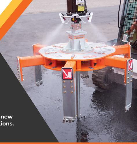
Mr. Manhole has developed a new misting system for our cutter tools, which will control silica exposure for your crews and allow you to fully comply with the new regulations.
