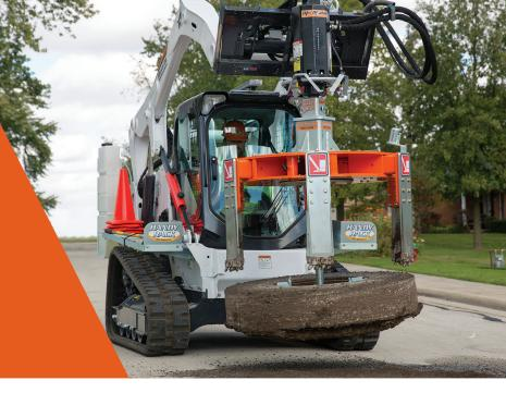
Our Cut, Pull, and Plate Package allows you to replace manhole frames temporarily with a steel plate then mill and pave right over them.
