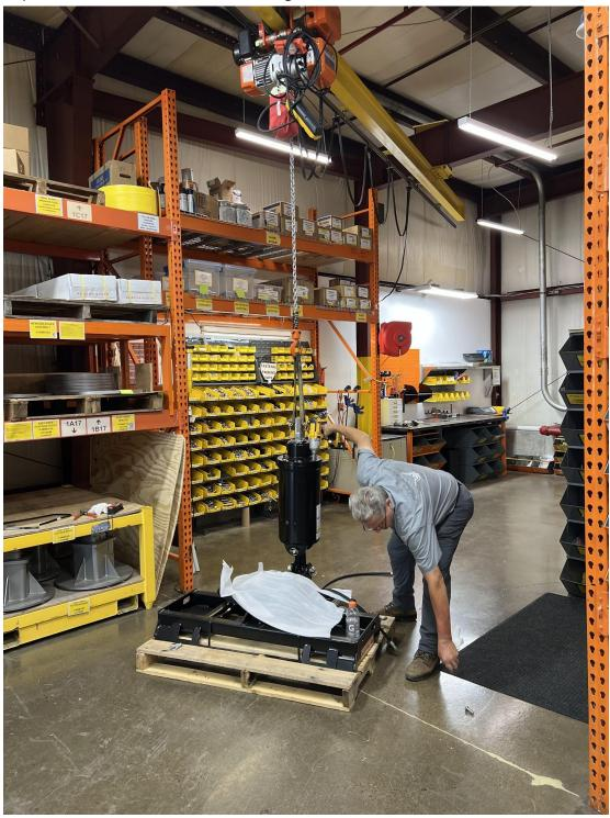
Carefully insert the internal motor and drive into the outer case taking care to protect the drain hose and fitting.
