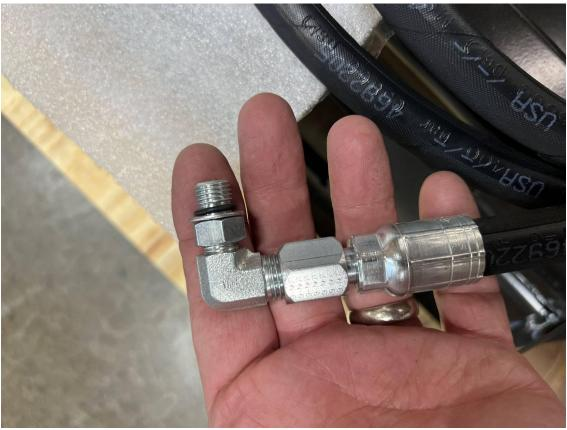
Install the drain hose on the 90 degree elbow fitting and route it through the outer case and out the bottom of the outer case.
