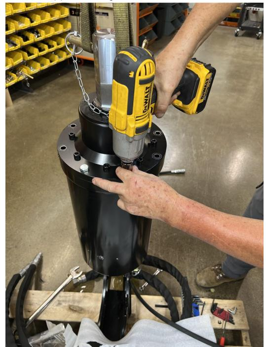
1. Remove the (8) bolts holding the motor internals to the outer case
